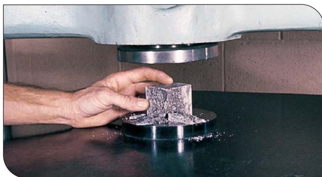
Fig. 2. Cube compressive-strength test. (IMG14091)
