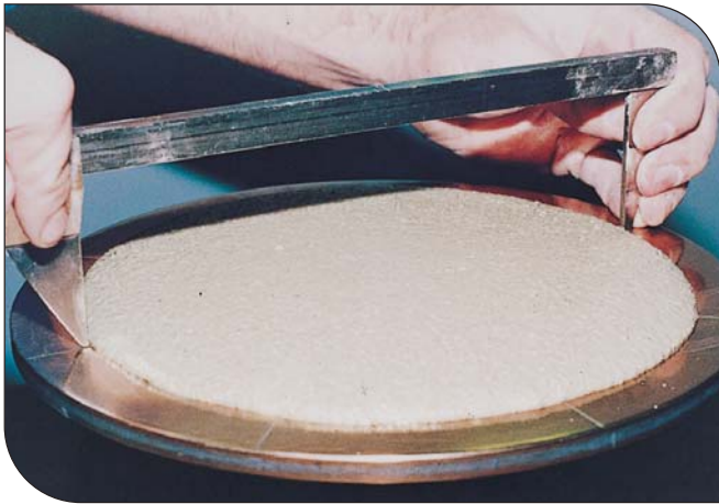
Fig. 5. Flow test. (IMG14093)
