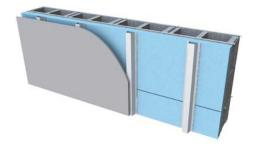
Continuous rigid insulation,  $1^{1}/_{2}$ -in. metal furring (for electrical rough-in) and  $1/_{2}$ -in. gypsum wallboard:
