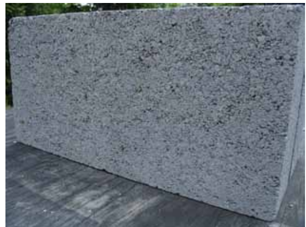
Figure 4—Photo Showing Surface Texture of Tested Units (ref. 7)
